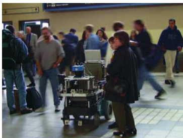
Fig. 10. The MAid automated wheelchair (left) relies upon the Velocity Obstacle approach for collision avoidance (right, source [8]).
